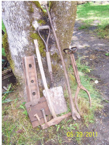
Photo 1. Angle Bar, Tie Plate, Spikes, Spike Maul, Shovel, Spike Bar, and Tie Tongs
