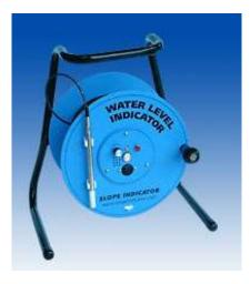
Current flows through the circuit when the end of the wire touches the water surface. Current is supplied by a small battery. To make a reading, lower the electric wire or sounding line until the needle deflects or the buzzer sounds.
